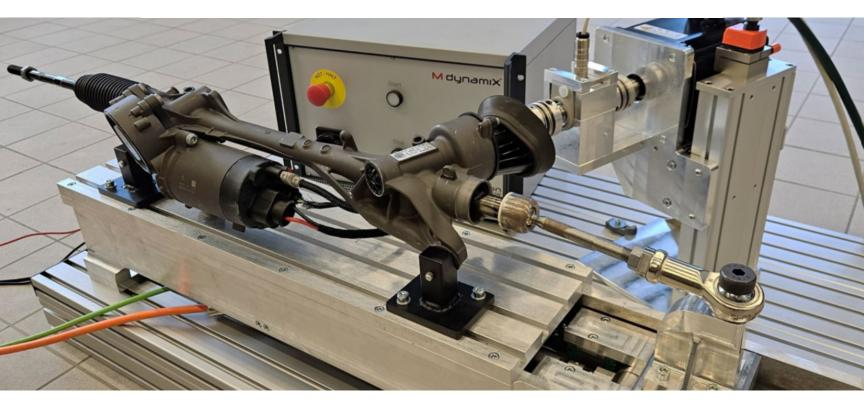
MXsteerHiL mini test bench allows for fully comprehensive testing of rack assist EPS with no performance compromises. With a maximum force of 16 kN and a maximum velocity of 300 mm/sec, the bench covers nearly all common steering tests within a footprint of only 1200 × 800 mm.
