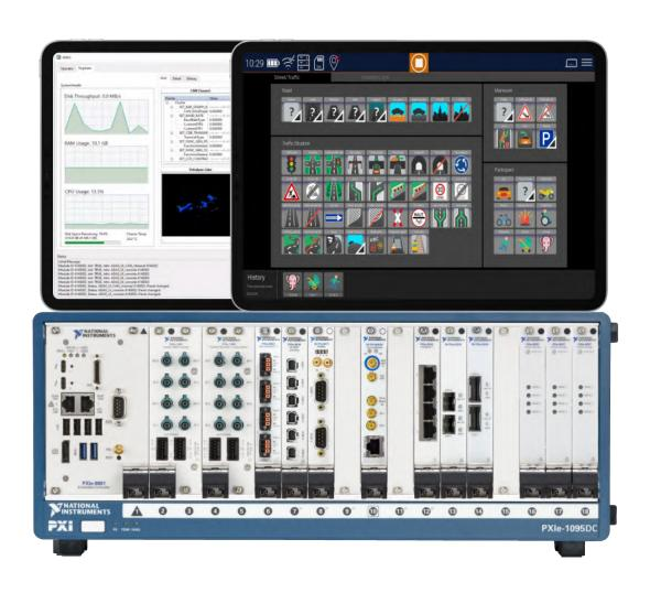
This ADAS Record System combines NI PXIe instrumentation, Seagate storage, and the NI/Konrad Data Record AD software. Konrad Technologies' Pre-Label Tool allows the user to collect and label the metadata during a drive test for a post event analysis. The user can pick from a library of the event labels or create custom labels and fields to locate specific data quickly. Configurations and drive scenarios can be stored and reused.
